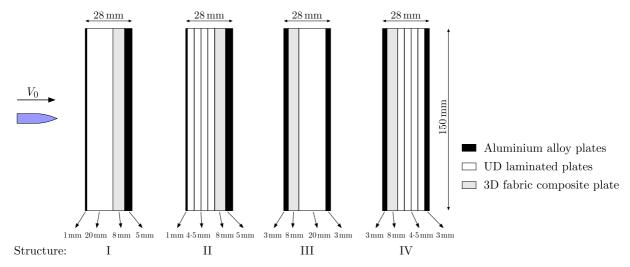
Fig. 2. Schematic of composite target plates
