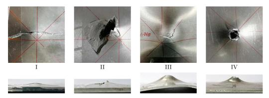
Fig. 6. Failure patterns of the rear panel of composite target plates
