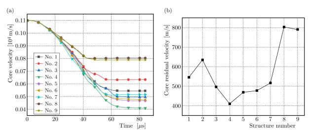
Fig. 12. Numerical simulation results: (a) time history curve of projectile velocity, (b) relation curve between the structure form and residual velocity
