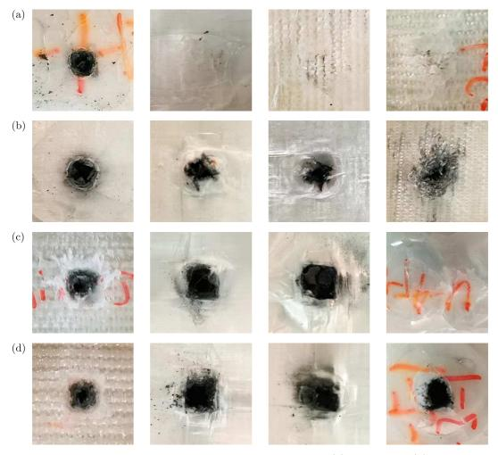
Fig. 7. Failure morphology of the core layer of each structure: (a) structure I, (b) structure II, (c) structure IV
