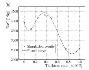
Fig. 13. (a) The relationship between EAC of different structures, (b) relationship between 3D fabric thickness ratio and EAC
