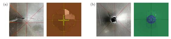
Fig. 10. Failure modes of the penetration test and numerical simulation: (a) structure I back plate, (b) structure IV back plate
