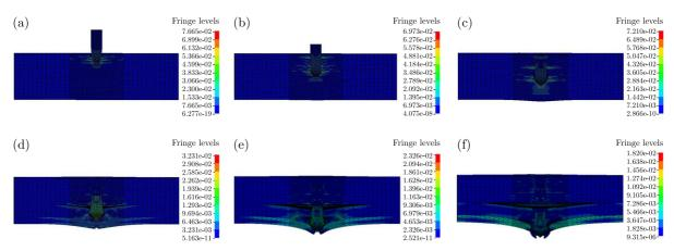
Fig. 11. Damage process of projectile penetration structure I: (a)  $t = 12 \,\mu\text{s}$ , (b)  $t = 20 \,\mu\text{s}$ , (c)  $t = 30 \,\mu\text{s}$ , (d)  $t = 45 \,\mu\text{s}$ , (e)  $t = 60 \,\mu\text{s}$ , (f)  $t = 70 \,\mu\text{s}$
